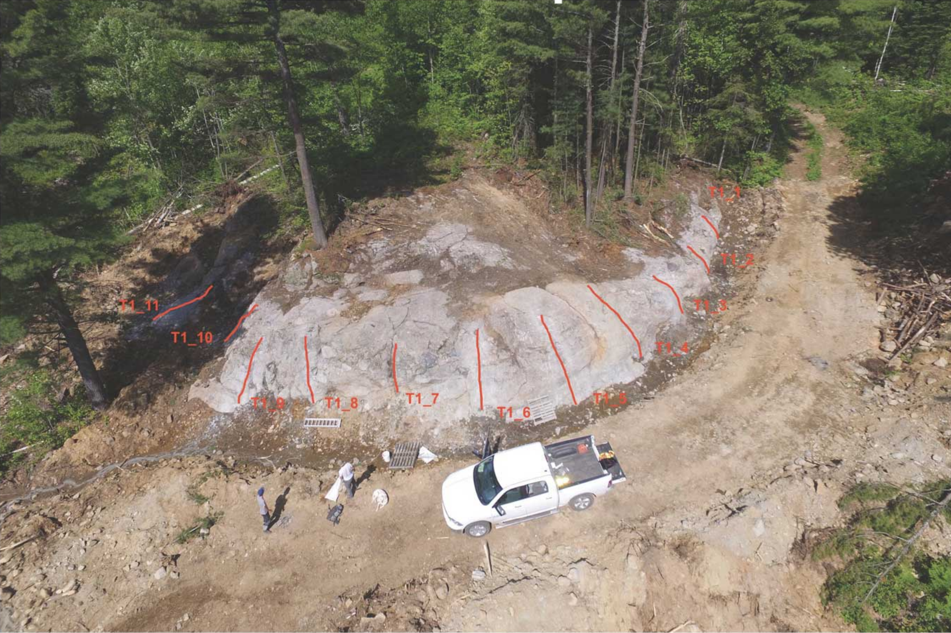
Figure 1 – Trench 1 Channel Sample and Proposed Bulk Sample Location
